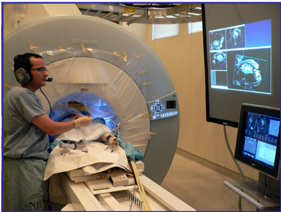
Fig. 1.6: Interventional cardiac MRI suite employing a modified clinical scanner with a shorter bore and a wider opening. Image courtesy of Elliott McVeigh, PhD, Johns Hopkins University, Baltimore, MD.
